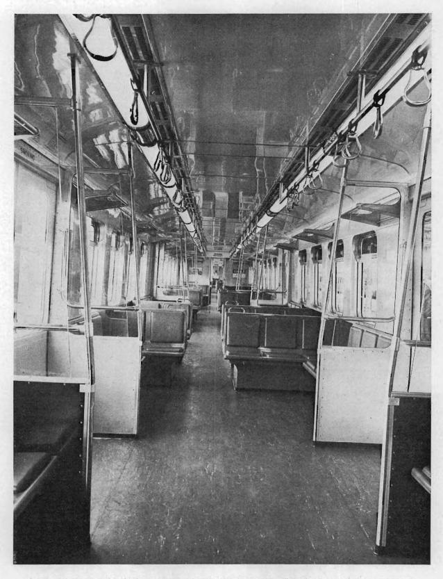
Interiors of the new 75 ft. suburban carriages with connecting doors open. The style of seating is common overseas.
